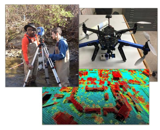
This course provides an opportunity for students to get hands-on experience in using UAVs, LiDAR, and GPS to obtain, process, and analyze geospatial data. It includes the field and lab components. The field component teaches students how to use the UAV, LiDAR, and GPS equipment to obtain data. The lab component teaches students how to process and analyze the data.
